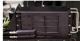
Liquid cooled sidewall chassis (>100W/slot) – Patent pending
